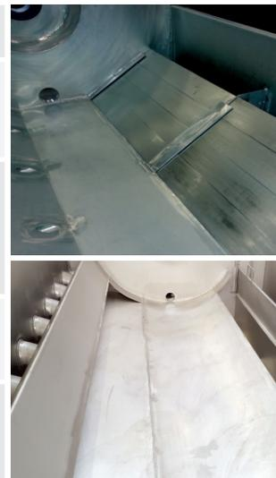
Note: All Tanks are manufactured in 304 St. St in thickness 3.0, 4.5 and 5.0 mm to suit the application.
